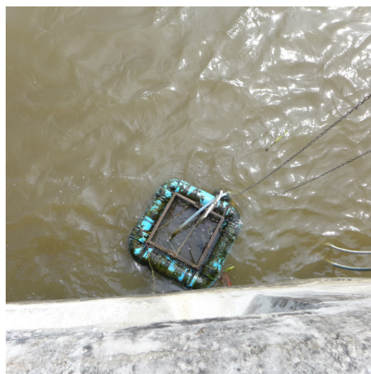
Water sampling site of a measuring station. The water is sampled by means of a submersion pump which is protected from debris and quick occlusion by a rough underwater metal cage. The sampling site is equipped with a float to allow water sampling during severely fluctuating water levels.
