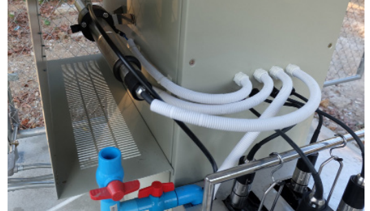
A spectral sensor with flow-through fitting, as well as additional compressed air cleaning, installed at the back of the measuring station.
