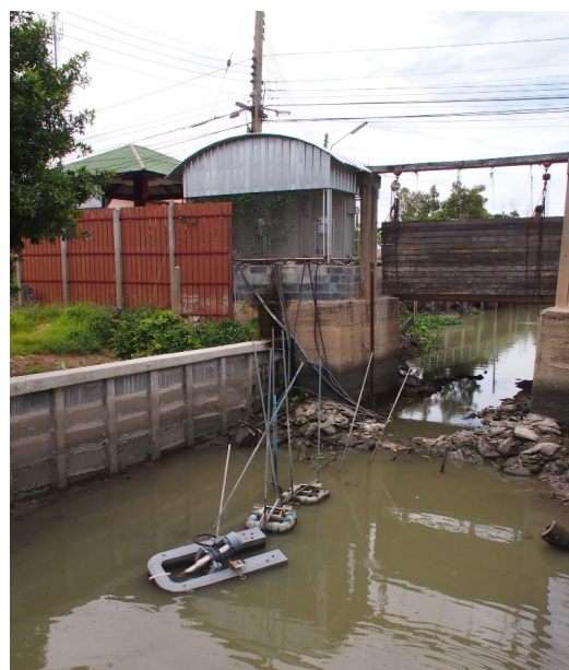
Khlong, where NiCaVis® 705 IQ tests for COD and nitrate were conducted by means of the spectral sensor. Discharged/inlet by a wastewater treatment plant in an industrial park in immediate vicinity.
